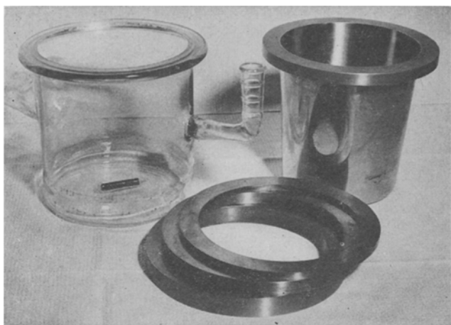
FIG. 1. Still pot for molecular distillation of waxes with metal head, brass washers, and magnetic stirring bar.
